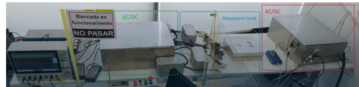
Complete Setup: Converters DC/DC, AC/DC, Resonant Chokes, Resonant tank- Capacitors, SST.
